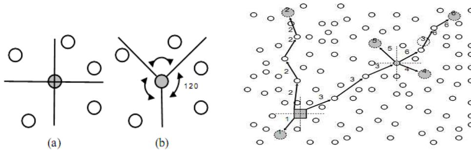
Figure 1 .a) dividing the space into four quadrants, and b) dividing the space into three 120 degree pieces
