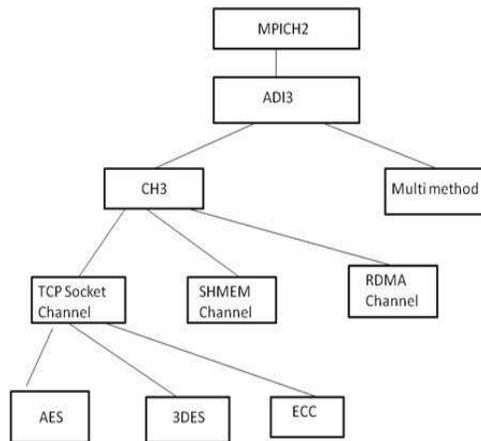
Fig 1. ES- MPICH2 implementation structure However, MPICH2 is not merely MPICH with MPI-2 extensions. It is based on a completely new design, aiming to provide more performance, flexibility and portability than the original MPICH2. The future development for MPICH, including those necessary to accommodate extensions to the MPI Standard now being contemplated by the MPI Forum.
