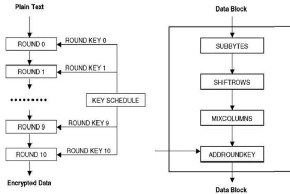
Fig 3 Internal operations of Advanced Encryption Standard
