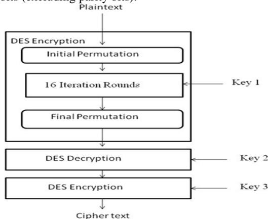
Fig 4 Internal operation of Triple Data Encryption Standard
