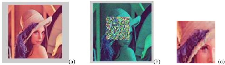
Figure 3. Image encryption experimental result 1: (a) Plain- image, (b) Selective Encrypted image (c) Selective decrypted image
