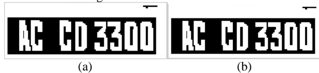
Figure 4.2: (a) Converted Black to white, (b) Connected component analysis
