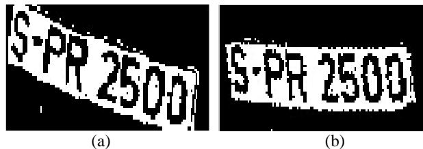
Figure 3.6: (a) Extracted plate, (b) Rotated plate
