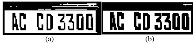
Figure 4.1: (a) Binarized number plate, (b) Erode image
