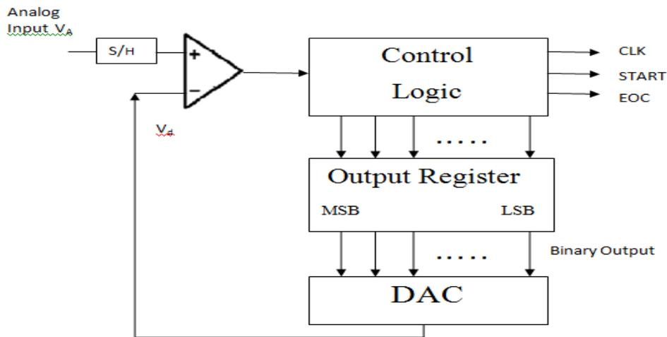
Fig : General Block Diagram of SAR ADC
