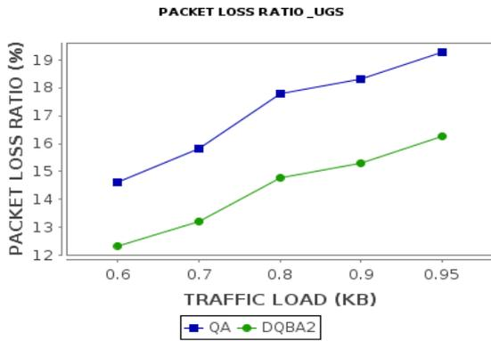
Fig. 6 Packet Loss Ratio of UGS traffic
