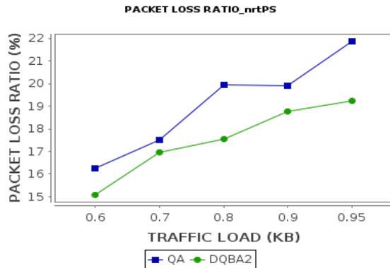
Fig. 8 Packet Loss Ratio of nrtPS traffic
