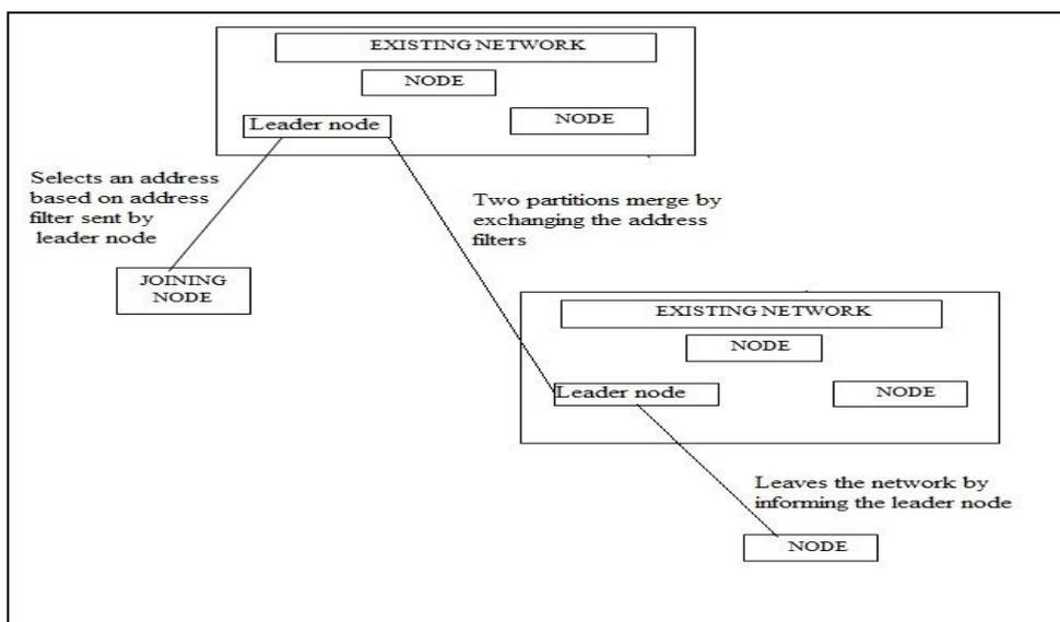
Fig. 3 System Architecture
