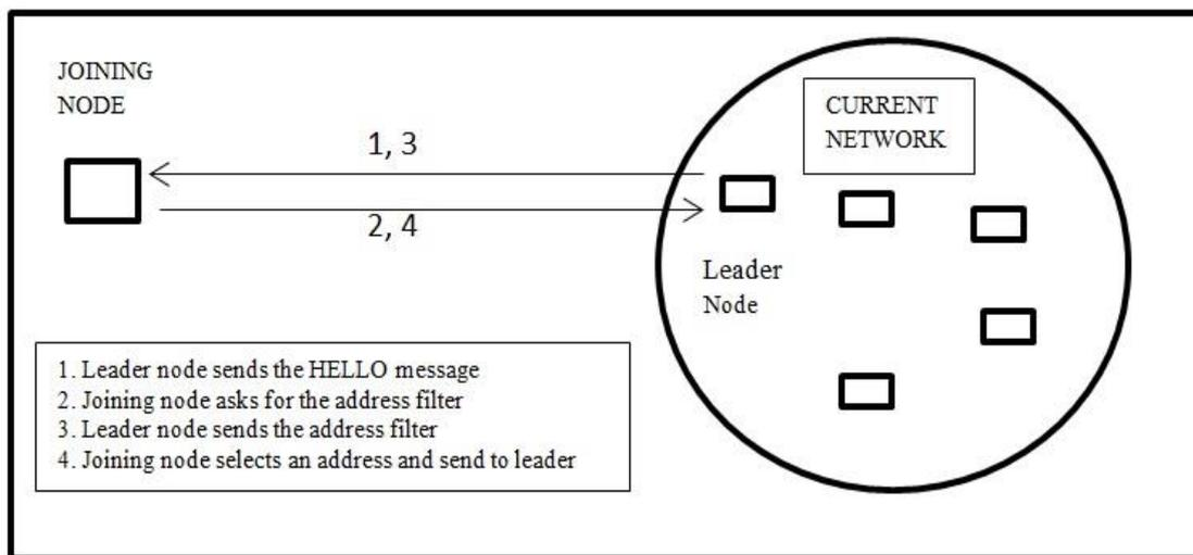
Fig. 1 Joining Node procedure
