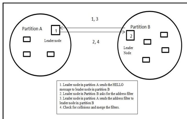
Fig. 2 Partition merging procedure
