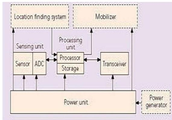
Fig 2.Components of sensor networks
