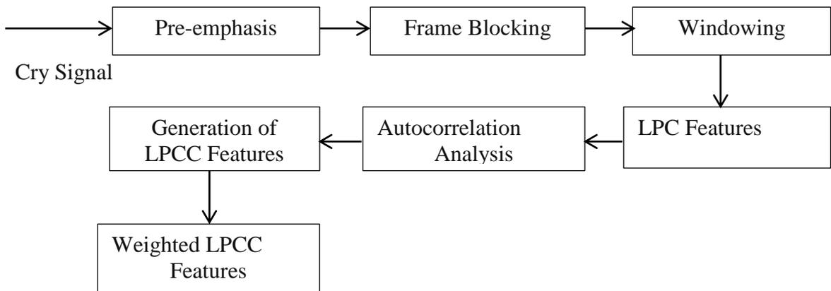
Fig.1. Block Diagram of the Feature Extraction
