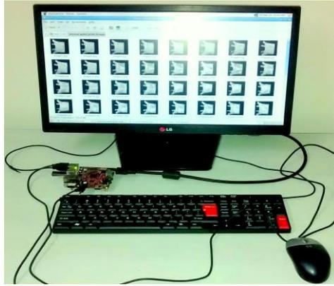
Fig.4. Beagleboard-xM setup for iris recognition system
