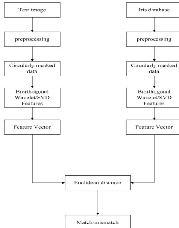
Fig.3.1. Block diagram of Iris recognition using Biorthogonal wavelet/SVD
