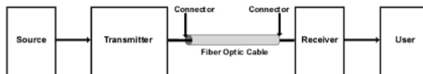
**Fig. 1 Block Diagram of Optical fiber communication.**
