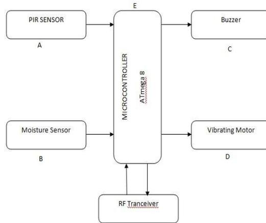
Fig 3 : Block diagram of the proposed system.
