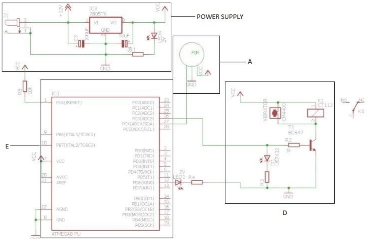
Fig 4 : Circuit Diagram of proposed system. The various sections have been marked corresponding to the block diagram.
