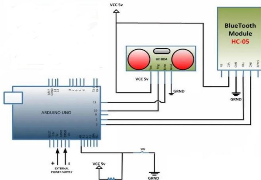
Figure 1: Architecture Diagram of the setup
