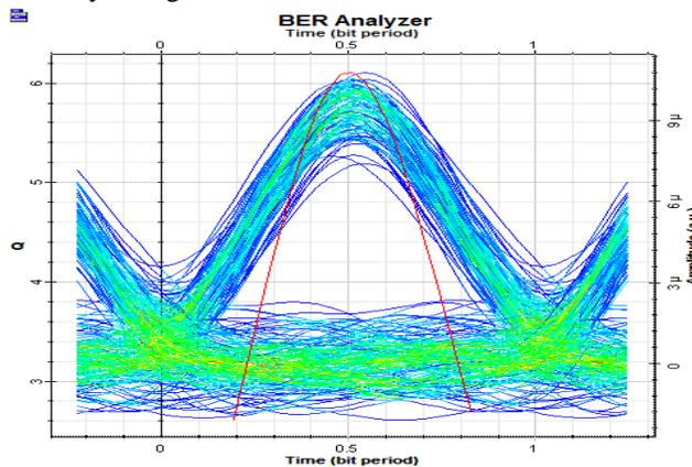
Fig 6. Eye Diagram of Upstream
