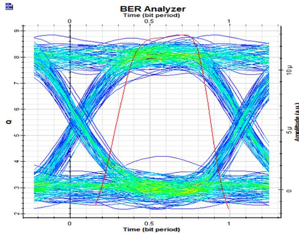
Fig 4. Eye Diagram of Upstream
