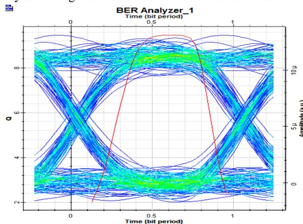
Fig 3. Eye diagram of downstream
