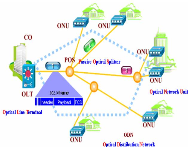
Figure 1 EPON Network Architecture
