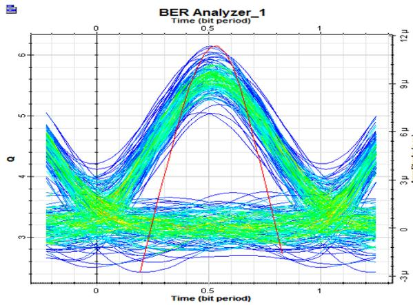
Fig 5. Eye diagram in downstream
