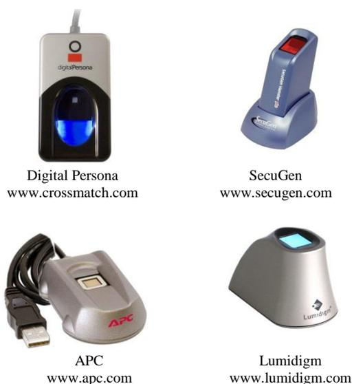
Fig. 5 Various Commercial Sensors Available for Live Capture of Fingerprints
