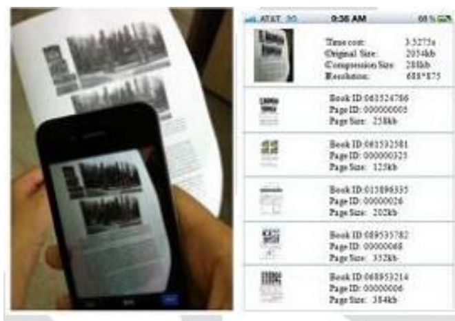
Fig 1: Right side shows the retrieved information from digital library Left side shows capturing the image by mobile device
