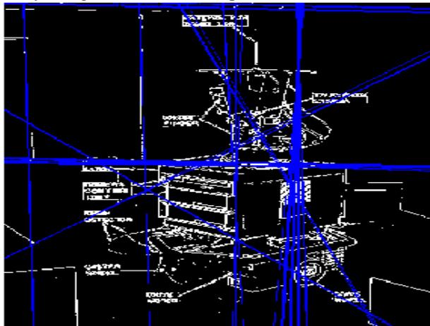
Figure 4: Finding lines using Hough Transform (adapted from [10])
