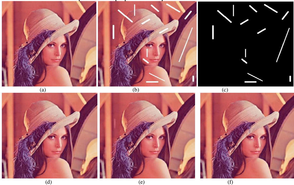
Figure 4 Inpainting of artificial lines on Lena's image. (a): Clean image. (b): Damaged by putting artificial lines. (c): Mask image. (d): Bertalmio's technique, PSNR= 49.765 dB and Exe. time=128.580 S. (e): FoE technique, PSNR= 45.6642 dB and Exe. time = 445.947 S. (f): Gaussian pyramid technique, PSNR= 50.6885dB and Exe. time= 2.625 S.
