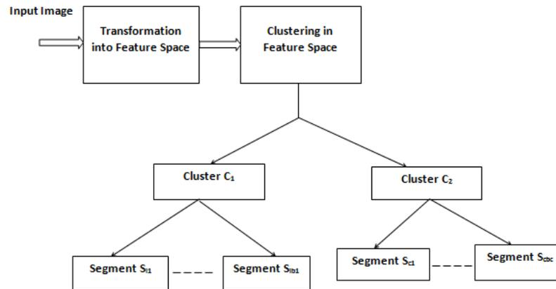
Fig. 2. Methodology of K-means Clustering method
