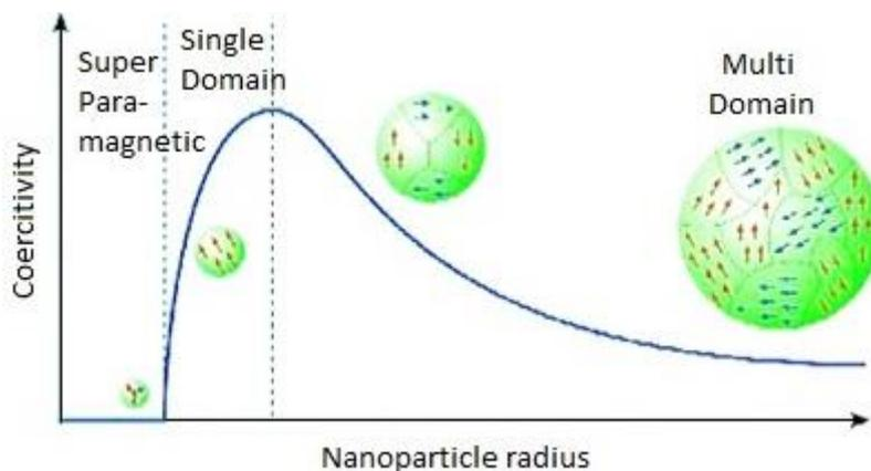
Fig 1: Figure of the relation between coercivity and nanoparticle radius. [2]
