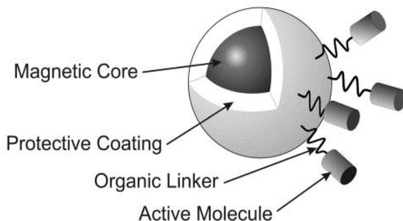
Fig 4. Structure of magnetic nanoparticle carrier [5]
