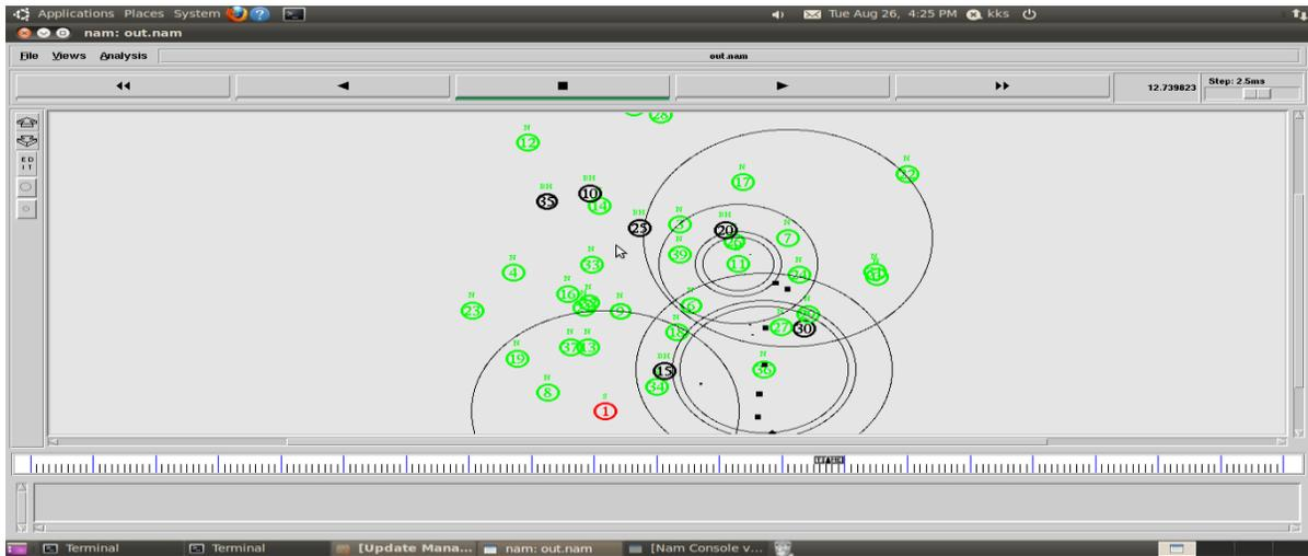
By introducing the malicious nodes, the packet drop can be done. The below simulation results show the packet drop in a manet when a black hole is implemented.
