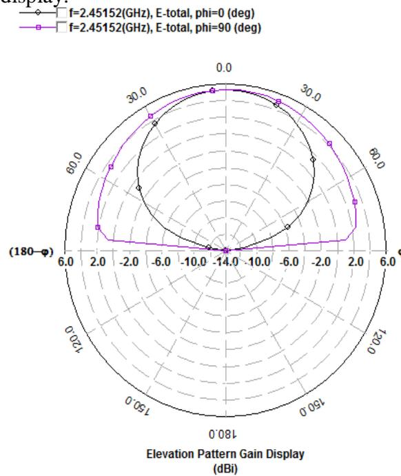
Fig.4(a) Elevation Radiation pattern of antenna at 2.45 GHz
