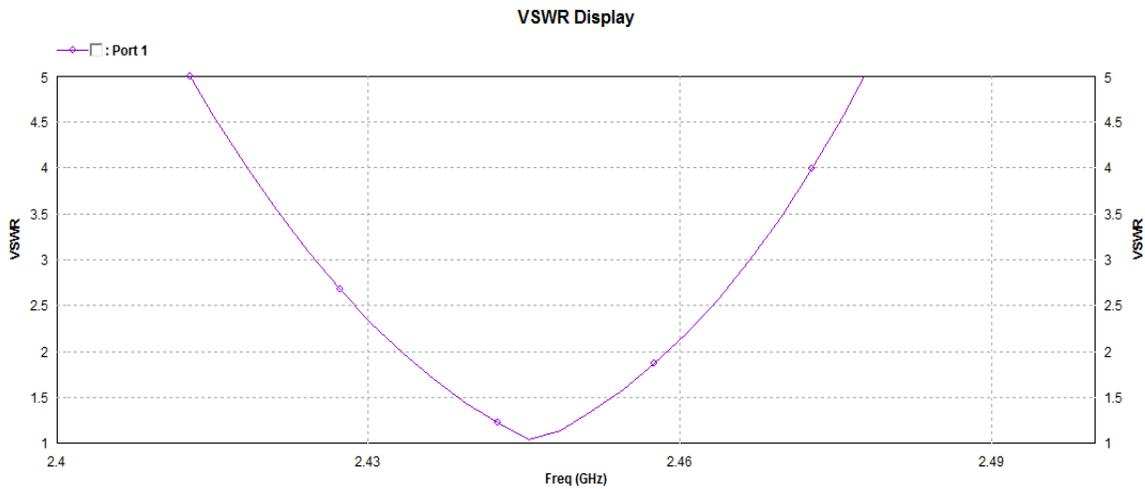
Fig.3 VSWR of antenna at 2.45 GHz frequency
