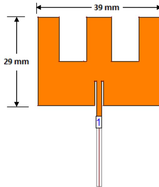
Fig.1 E-shape patch antenna
