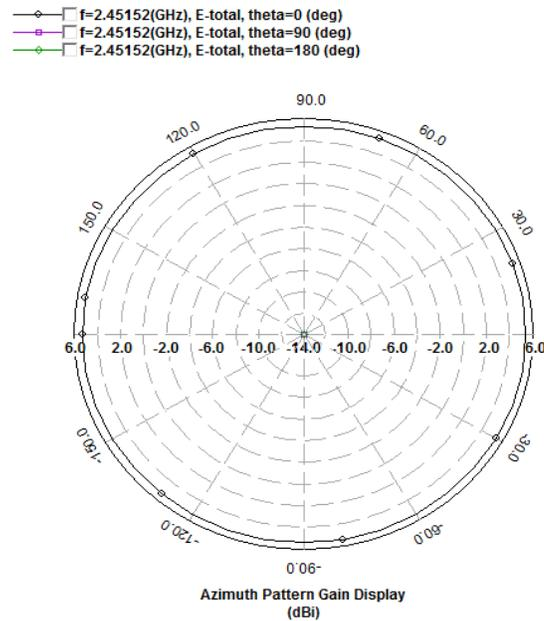
Fig.4 (b) Azimuth Radiation pattern of antenna at 2.45 GHz
