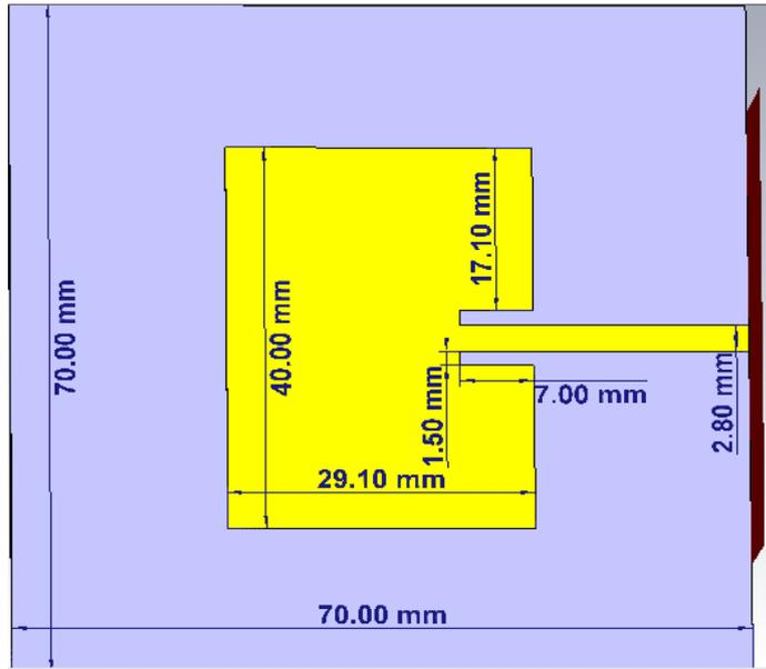
Fig.1 Inset feed microstrip patch antenna
