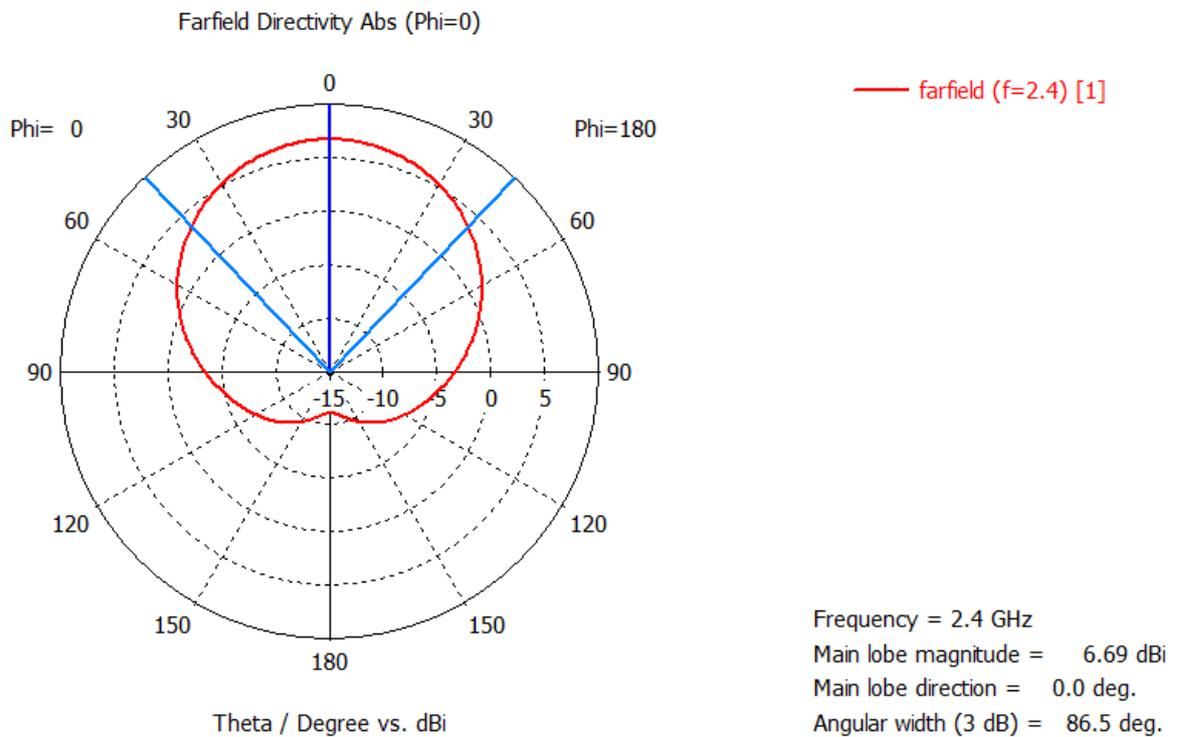
Fig.4 Radiation pattern of antenna at 2.4 GHz and  $\phi = 0$  degree
