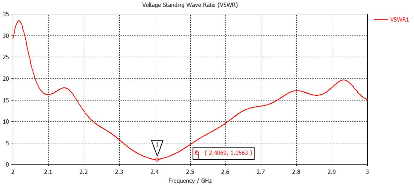
Fig.3 VSWR of antenna at 2.4 GHz frequency
