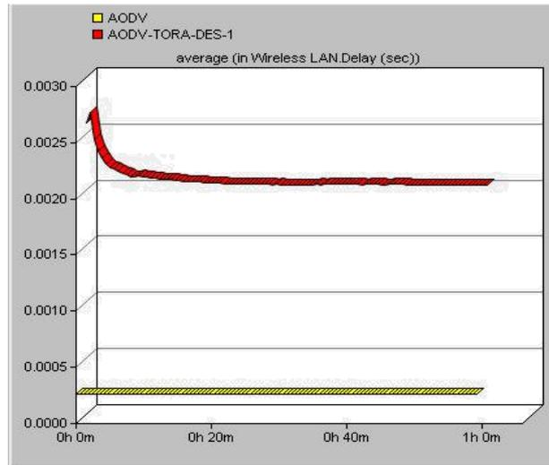
Fig 4.Delay for AODV and TORA
