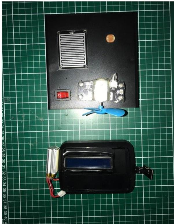
Fig. 2. Outdoor and Indoor Parts of our Weather Station.
