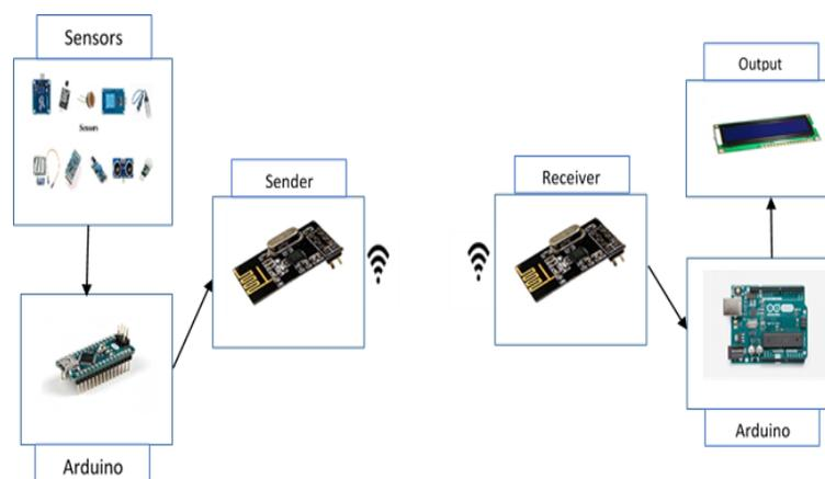
Fig. 1. Weather Station Structure.
