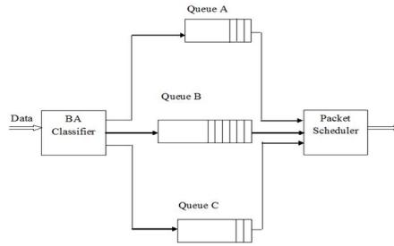
Figure 2.1: The structure of a DS core router
