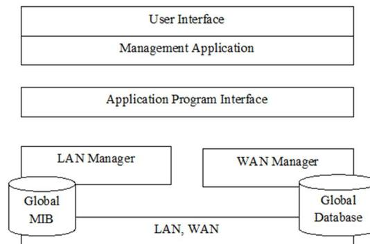
Fig. 4.4. Configuration of the integrated network management system
