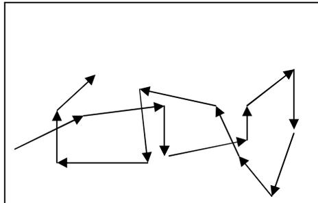
Fig3. Random Walk Mobility model example node movement
