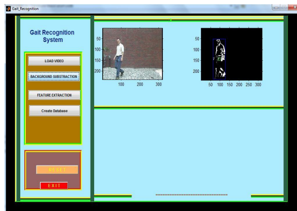
Figure 8. The input video is loaded and background subtraction is performed.
