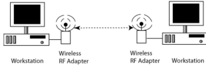
**Figure 2.1:**Point to Point Connection
