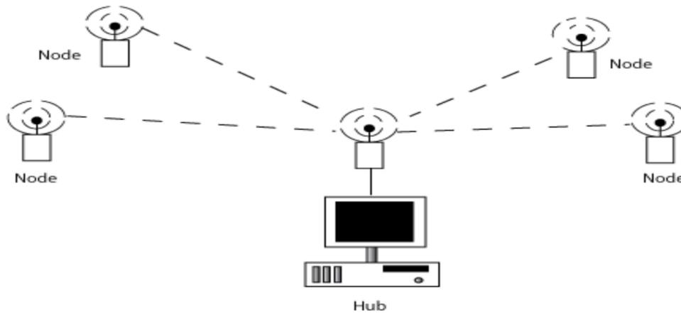
**Figure 2.2:**An example of a star network topology would be a Wi-Fi network where the access point is the hub and a laptop may be a node. It shows star network topology.
