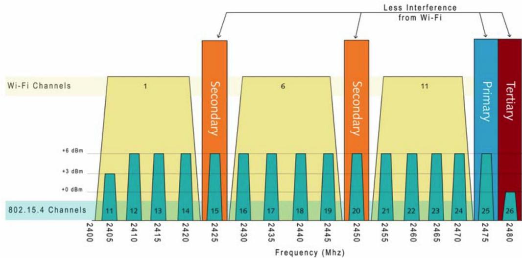
**Figure 3.2:** A comparison between the IEEE 802.14.5 RF channels and common Wi-Fi RF channels.
