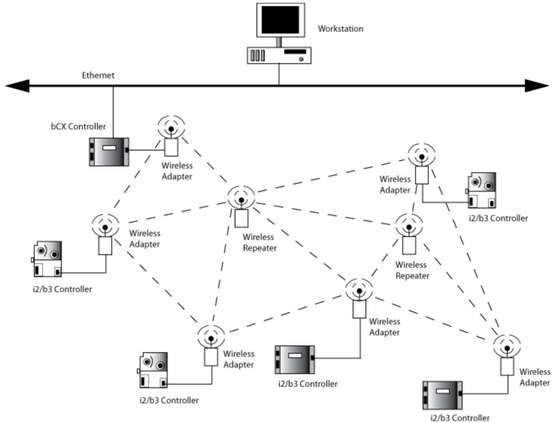
**Figure 1:** Wireless repeaters and links in a typical Andover Continuum mesh network
