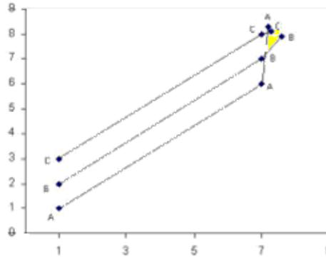
**Fig 4:** Movements of three Mobile Nodes using the Column Mobility Model
