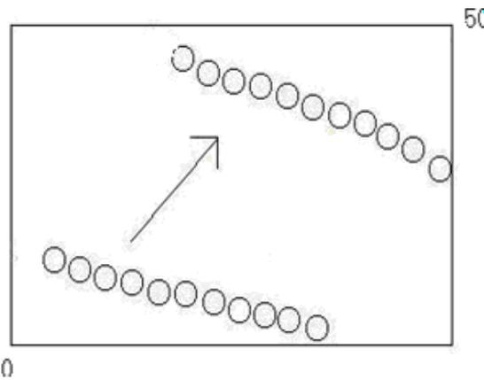
**Fig 5:** Traveling pattern of 11 Mobile Nodes using the Column Mobility Model
