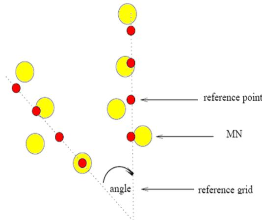
**Fig 2.** Movements of three Mobile Nodes using the Column Mobility Model
