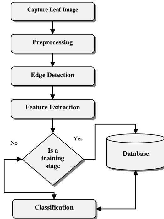
Fig. 2 The main block diagram of proposed system.
