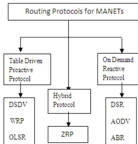
**Figure 2.1.** Different types of Routing protocols in MANETs
