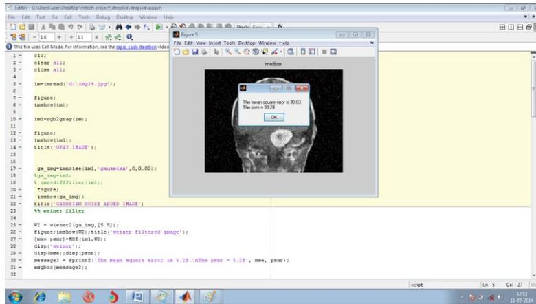
The above figure shows median filter added to noisy image.
