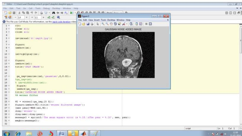
The above figure shows Gaussian noise added image
