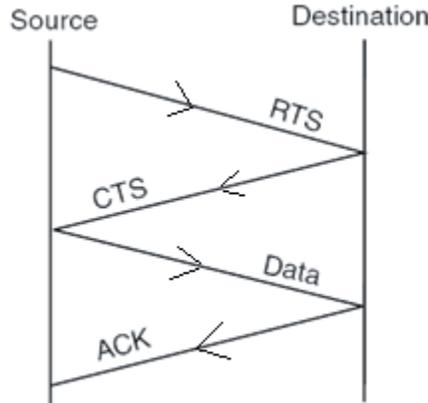
Figure 1 : Four Way Handshaking (DCF)
