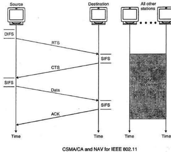
Figure 2 : CSMA/CA Mechanism
