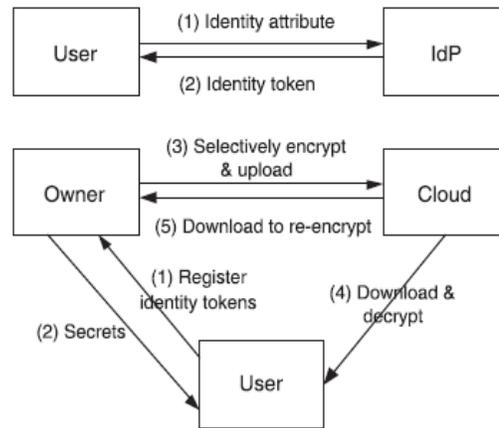
**Figure 3: Overall System Architecture**
