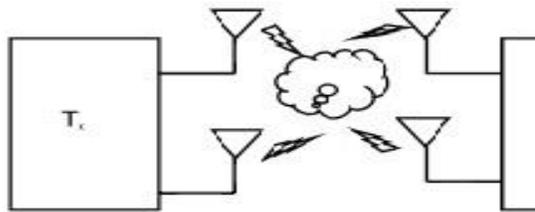
Fig.1.1 Basic Structure of MIMO
