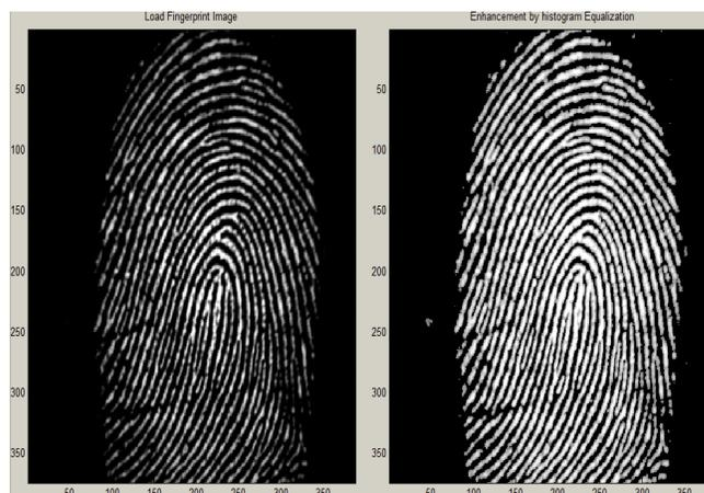
Fig 6. Histogram Equalization of fingerprint image
