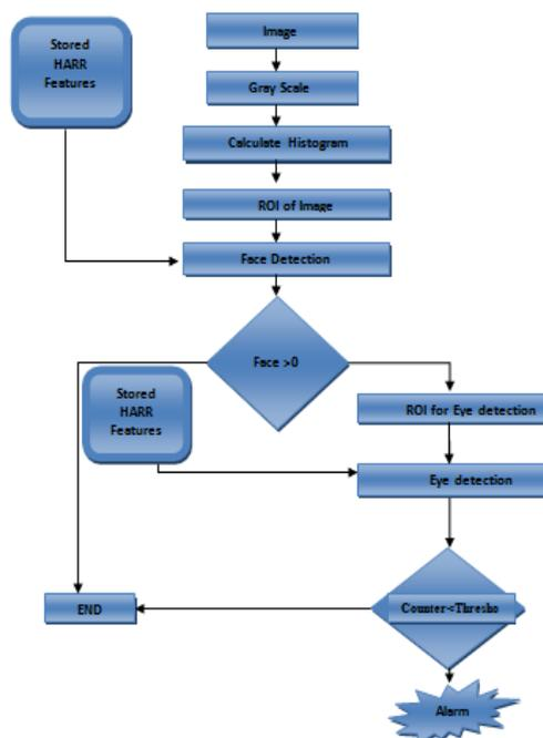
**Figure 2:** Flow chart of Purposed System
