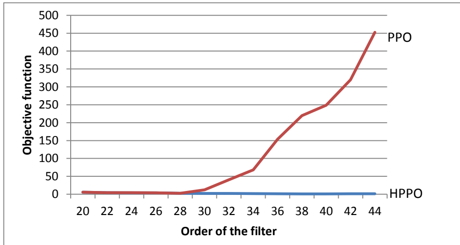
Fig 1: Comparison of objective function of HPPO and PPO for different filter orders
