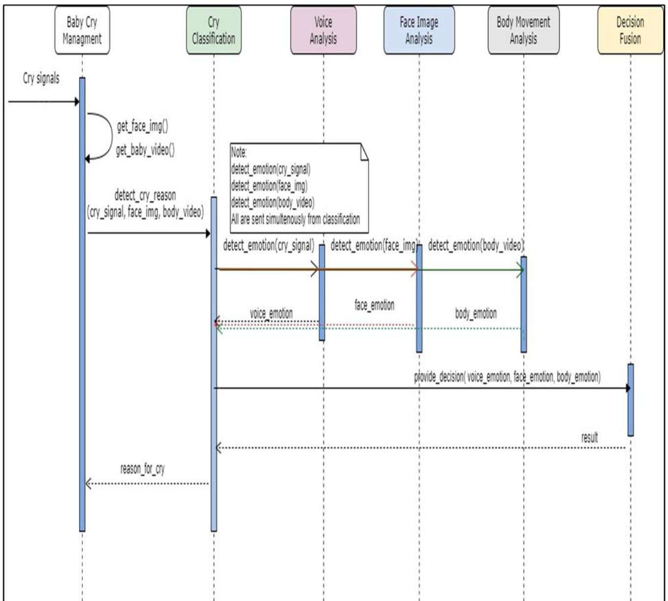
Fig. 6 Cry classification sequence diagram
