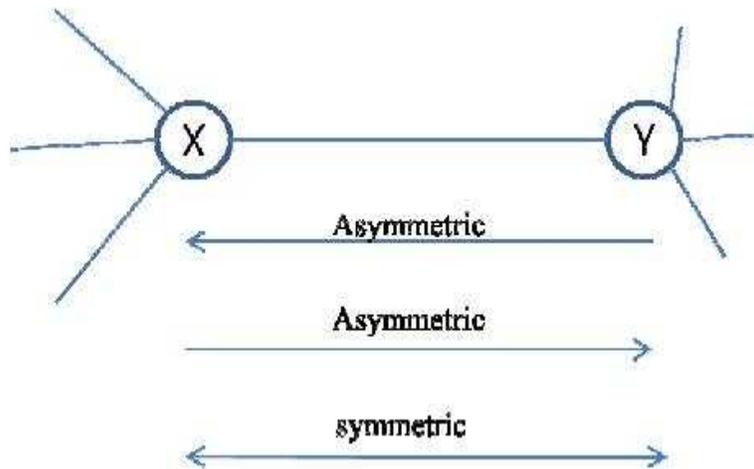
Fig. 1 HELLO messages in MANET using OLSR algorithm
