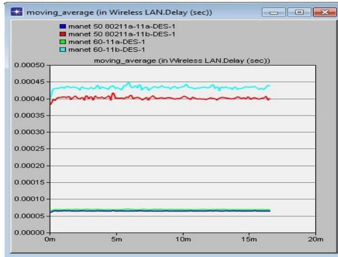
Fig 3 End to end network delay
