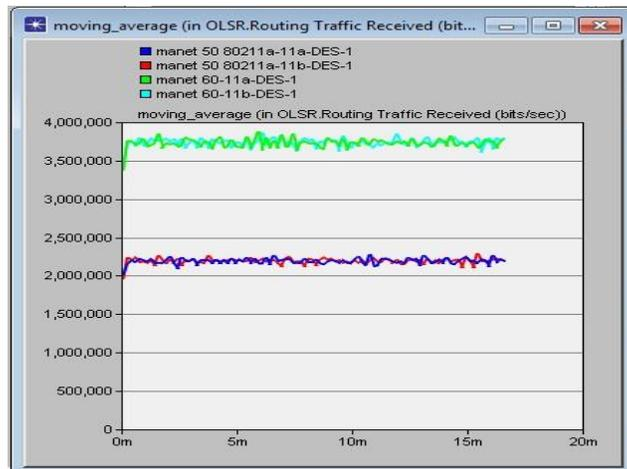
Fig 6 OLSR routing traffic received
