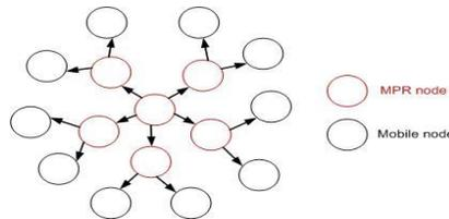
Fig. 2 Flooding Packets using MPR
