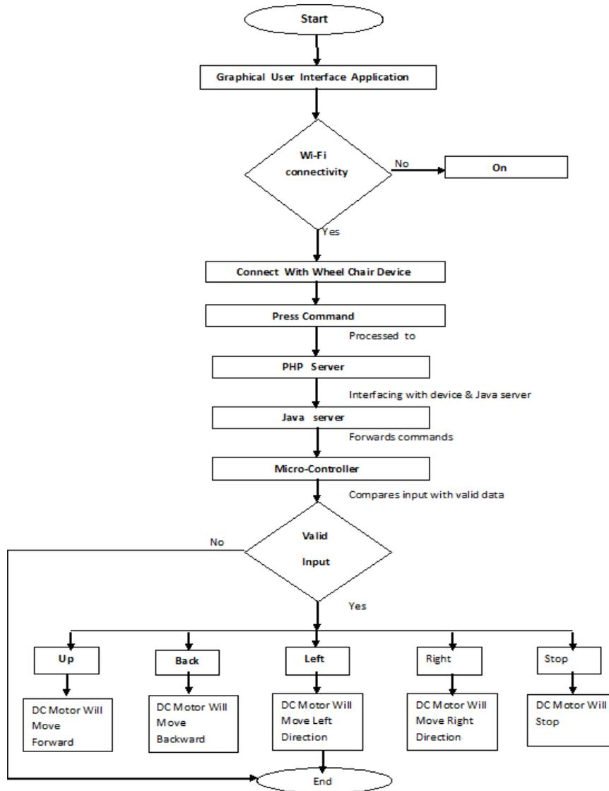
Fig 5: Flowchart for GUI Command
