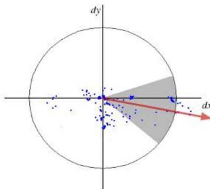
For feature description, SURF uses Wavelet responses in horizontal and vertical direction (again, use of integral images makes things easier). A neighborhood of size  $20s \times 20s$  is taken around the keypoint where  $s$  is the size. It is divided into  $4 \times 4$  subregions. For each sub region, horizontal and vertical wavelet responses are taken and a vector is formed like this,
