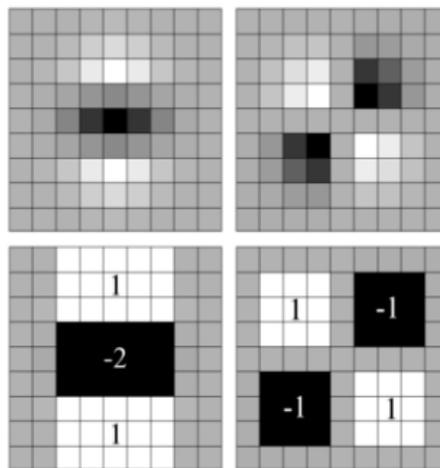
Fig 2.3:  $L_{yy}(\mathbf{x}, \sigma)$  and  $L_{xy}(\mathbf{x}, \sigma)$  Discretized Gaussians and the approximations  $D_{yy}$  and  $D_{xy}$
