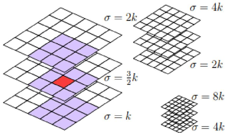
Fig. 2. 2 octaves with 3 levels, the neighborhood for the 3x3x3 non-maximum suppression used to detect features is highlighted
