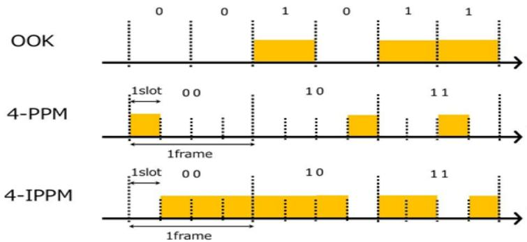
Fig. 3 inverse pulse position modulation 4-PPM
