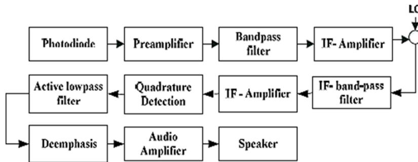
Fig. 5 the block diagram of underwater communication receiver
