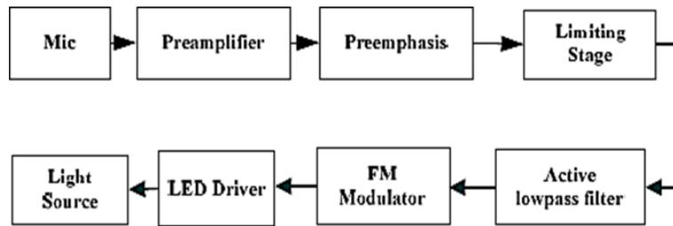
Fig. 4 the block diagram of underwater communication transmitter
