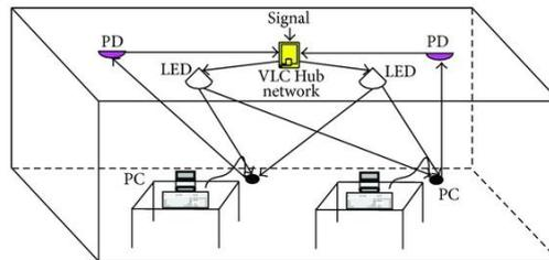
Fig. 1 A schematic diagram of an indoor visible light communication
