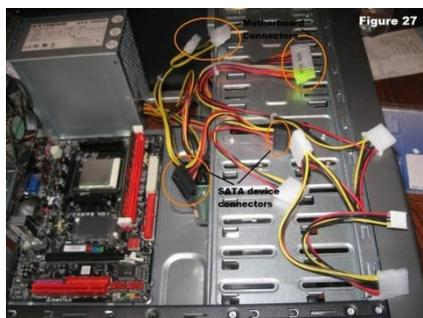
Fig 14: Connect Cables
