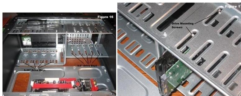
Fig 7: Install Hard Drive
