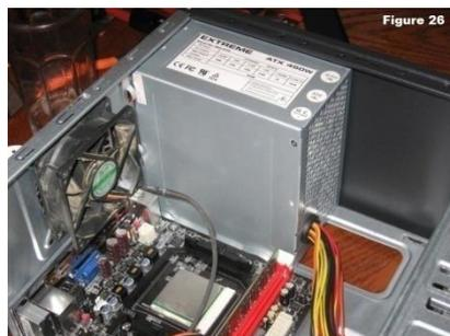
Fig 13: Install Power Supply
