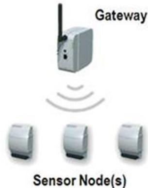
Fig. 1 A WSN Component, Gateway and Distributed nodes
