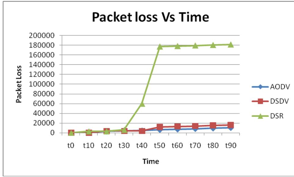
Fig 5 Packet loss Vs Time
