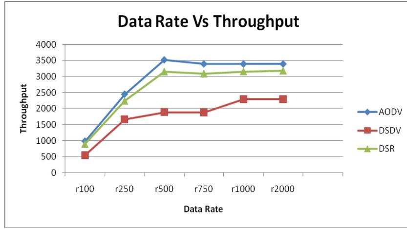
Fig. 3 Data Rate Vs Throughput
