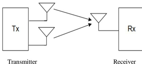
Fig 5. MISO antenna configuration
