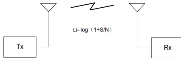
Fig 2. SISO wireless channel system
