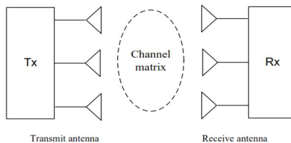
Fig 3. MIMO wireless channel system
