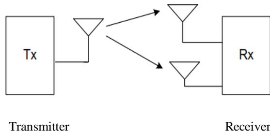
Fig 4. SIMO antenna configuration
